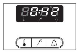
After a certain time the estimated **residual time** (i.e. the time left to run), appears in the oven display. The actual core temperature is no longer visible and cannot be called up.
